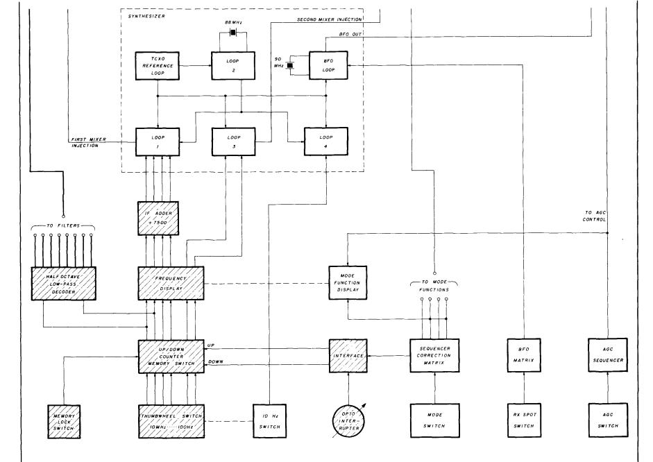
fig. 2. Areas of the transceiver discussed in this article. The block diagram shows the half-octave automatic filter system, which provides attenuation for harmonics generated by the wide-band transmitter. Low-pass filters are switched in along with bandpass filters. Total passband ripple does not exceed 0.1 dB.
